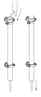
Pull precisely and with caution at the power cord to ensure a tight fitting of the two lamp parts
