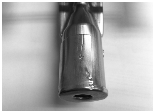
Burner Set at NG
