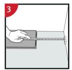
At the end of the first row, put a spacer to the wall and measure the length of the last panel to fit.
