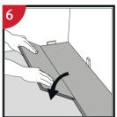
Place the plank and angle against the plank in the previous row, press forward and fold down at the same time. Leave the plank in a somewhat up angled position when the planks start to lock. To make this easier, a wedge with the suitable angle can be placed under the plank near the short side joint as support.
