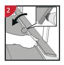
Remove the vertical locking part of the strip with a chisel, put applicable glye on the strip and push the panels horizontally together. Place some spacers between last board and the wall.
