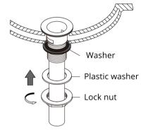
Install washer, plastic washer and lock nut onto pop-up body from underneath the basin. And then tighten lock nut.
