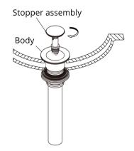
Put stopper assembly into drain.
