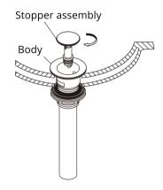
Put stopper assembly into drain.
