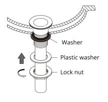
Install washer, plastic washer and lock nut onto pop-up body from underneath the basin. And then tighten lock nut.
