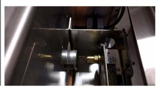
INCORRECT INSTALLATION THE ORIFICE IS OUT OF POSITION AND IS NOT INSERTED INTO THE VENTURI
