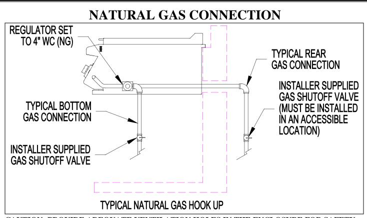
CAUTION: PROVIDE ADEQUATE VENTILATION HOLES IN THE ENCLOSURE FOR SAFETY PURPOSES IN THE EVENT OF GAS LEAK.
