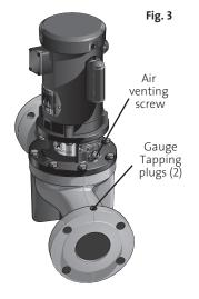
All air in the pump and suction line must be purged before starting the pump.
