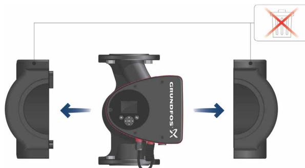
Fig. 3 Fitting insulating shells to the pump
