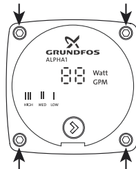
Fig. 4 Remove the four socket head cap screws on the power head to change the power head position
