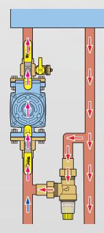
Under partial loads, the DPBV opens to ensure quiet operation and appropriate pressures at the boiler circulator. With all zones active, the DPBV remains closed
