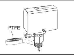
**c.** Insert the flow switch into the pipe tee. Turn the flow switch two (2) or three (3) revolutions clockwise until tight. Do not put excessive force on cover when turning.
