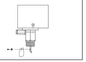
**b.** Apply pipe sealing compound or PTFE tape to the flow switch pipe threads.
