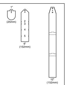
**a.** Trim paddle by cutting at appropriate notch with non-serrated tin snips.
