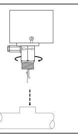
d. Place a 1 3/4" open end box wrench on flow switch body to tighten to final position. Final position is with arrow on body aligned in the same direction as liquid flow.
