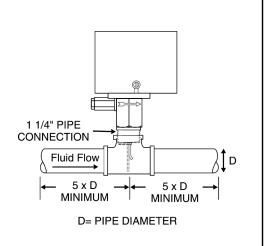
a. The flow switch must be installed in the pipe using a threaded tee connection or welding fitting of minimum length such as a half coupling. Use a face or hex bushing to reduce the tee outlet to 1 1/4" pipe thread if a reduced tee outlet thread size fitting is not available.
