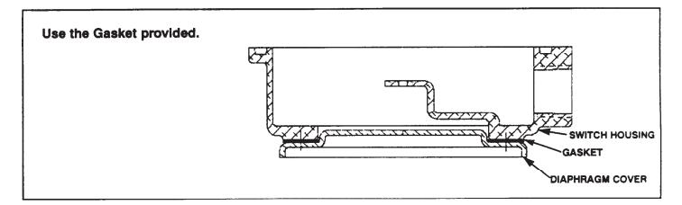
IMPORTANT: Do not use both the O-Ring and the Gasket for seal replacement. Using both will prevent the Flow Switch from operating.
