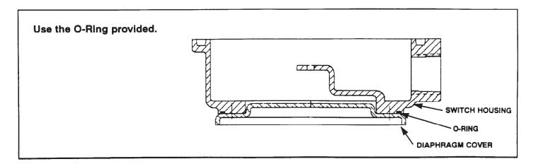
For Models with a Flat Surface Switch Housing:
