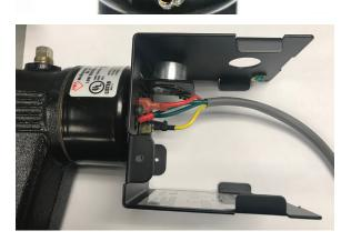
Install new e-11M switch enclosure using existing screws or ones provided with control kit.
