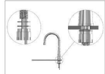
3. Attach the counter weight to the pull out flexible hose (part 2) DO NOT TIGHTEN (as the counter weight will need to be adjusted later on. Connect the flexible hoses and tighten (part 7) to the water outlet ensuring the rubber seal is not missed.
