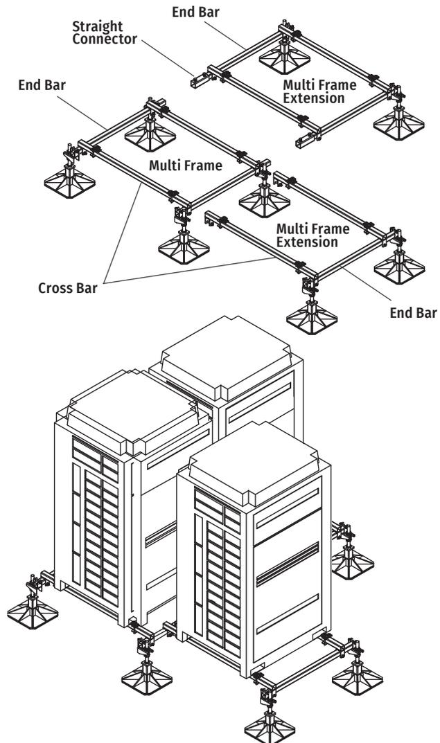
**NOTE:** Designed for heavy loads without penetrating the roof. Allowable foot pressure will be subject to roof build-up, typically detailed by a structural engineer. Cross bar spacings are adjustable to accommodate various unit sizes.
