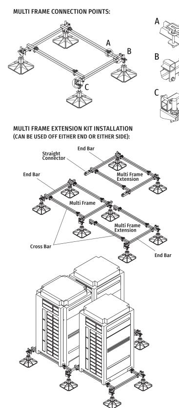
**NOTE:** Designed for heavy loads without penetrating the roof. Allowable foot pressure will be subject to roof build-up, typically detailed by a structural engineer. Cross bar spacings are adjustable to accommodate various unit sizes.
