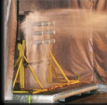
After test burns, assemblies are immediately subjected to a hose stream test to complete the ASTM E-814 (UL 1479) or ASTM E-1966 (UL 2079) procedure.
