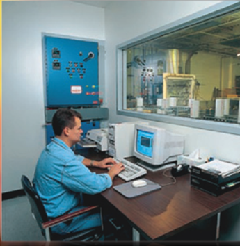
A computerized control room monitors all phases of test burns as specified by ASTM E-814 (UL 1479) or ASTM E-1966 (UL 2079).
