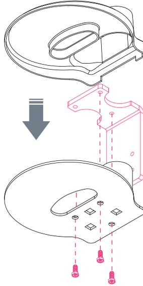
Insert carriage bolt between base covers and clamp shut. Remove backing from adhesive and adhere to bottom of base. Insert bolt from base into grommet and secure with hardware.
