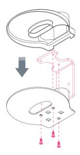
Insert carriage bolt between base covers and clamp shut. Remove backing from adhesive and adhere to bottom of base. Insert bolt from base into grommet and secure with hardware.
