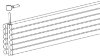
Using a hammer & steel rod to remove the centre block piece
