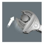
With its automatically and continuously gripping parallel jaws the Joker spanner 6004 covers all dimensions in the respective field of application. The tool automatically finds the required size when placed on the bolt or screw, no setting required.
