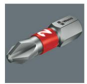
BiTorsion bits are absolutely premium products. They have a BiTorsion zone softer which reduces the hardness of the shaft by about 20 % in comparison to the drive tip. This means that the peak loads that cause bit breakage and premature wear are absorbed in this zone - something which enhances the service life of the bits.
