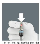
adaptor without moving the sleeve. The lock is activated automatically as soon as the bit is applied to the screw. Bits are held securely and wobble-free.
