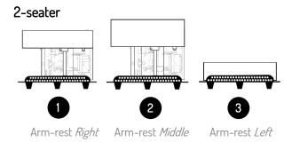
A two-seater Bio Wash is packed on three pallets.
