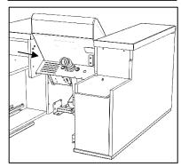
3. Connect "Arm-rest *Middle"* to the metal parts of "Arm-rest *Right"* with the countersunk bolts
