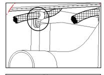
23. Secure water pipes at the correct side
