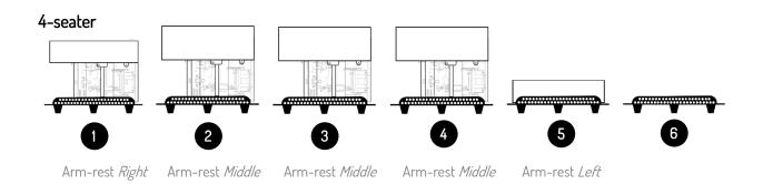
A four-seater Bio Wash is packed on six pallets.
