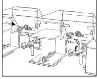
7. Connect "Arm-rest *Middle*" to the metal parts of "Arm-rest *Middle*" with the countersunk bolts
