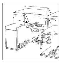
12. Connect "Arm-rest *Left*" to the metal parts of "Arm-rest *Middle*" with the countersunk bolts
