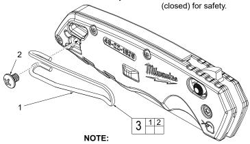
Apply a drop of non-permanent thread locking sealant (Loctite  $^{\circledR}$  222 or the equivalent) to the thread of screw #2 prior to installation.
