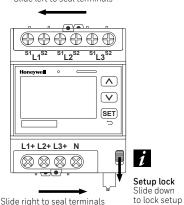
Max. diameter for power cables 0.75 mm2 to 2.5 mm2 / AWG14 to AWG18 at maximum 0.8 Nm.
