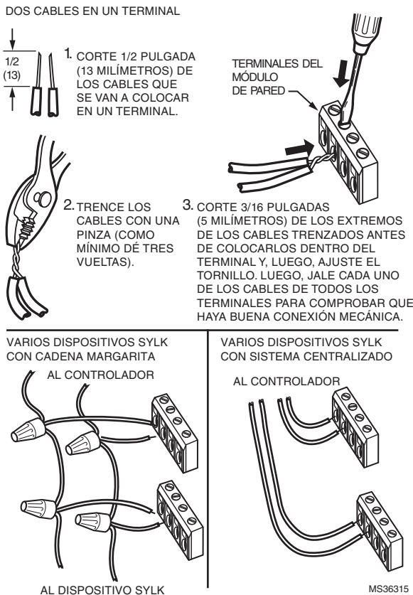
Fig. 6. Options for wiring multiple Sylk devices.
