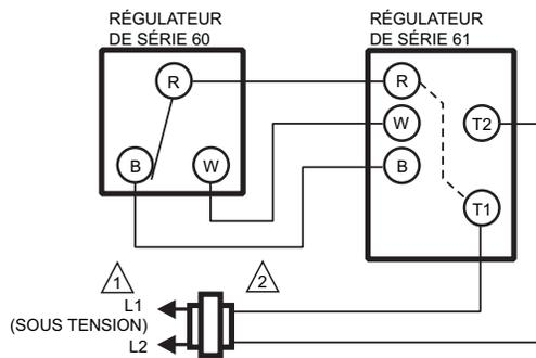
⚠ ALIMENTATION. FOURNIR, AU BESOIN, UN DISPOSITIF DE COUPURE ET UNE PROTECTION CONTRE LES SURCHARGES.
