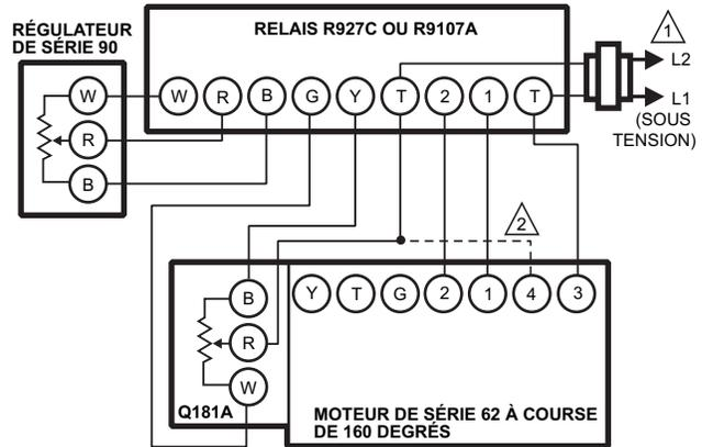
⚠ ALIMENTATION. FOURNIR, AU BESOIN, UN DISPOSITIF DE COUPURE ET UNE PROTECTION CONTRE LES SURCHARGES.
