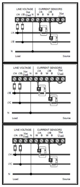
Use the diagram that corresponds to the existing circuit(s) being monitored.
