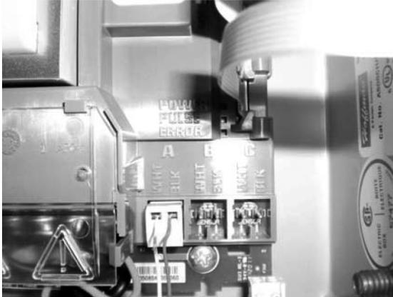
**Fig. 10. Sensor Polarity.** When current sensor is installed properly, error LED is off. If the Error LED is illuminated, then disconnect the gray plug and reverse the input lead. If it clears, the “Sensor Error” then mark appropriately. Repeat for all sensors.
