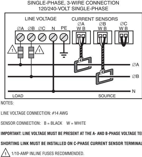
**Fig. 8. Single-Phase, 3-Wire Connection 120/240-Volt Single-Phase.**
