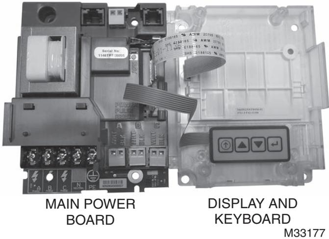
**Fig. 1. Main Power Supply Board & Display Board.**
