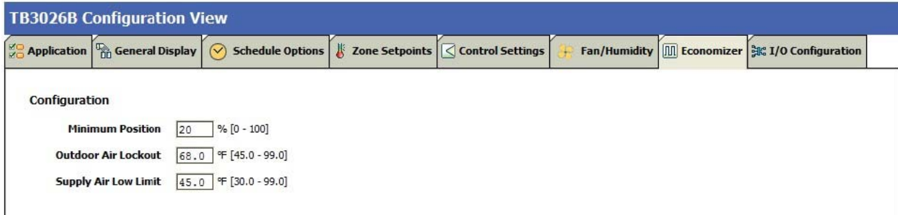
Fig. 79. Economizer Screen (Four Pipe Fan Coil Unit)
