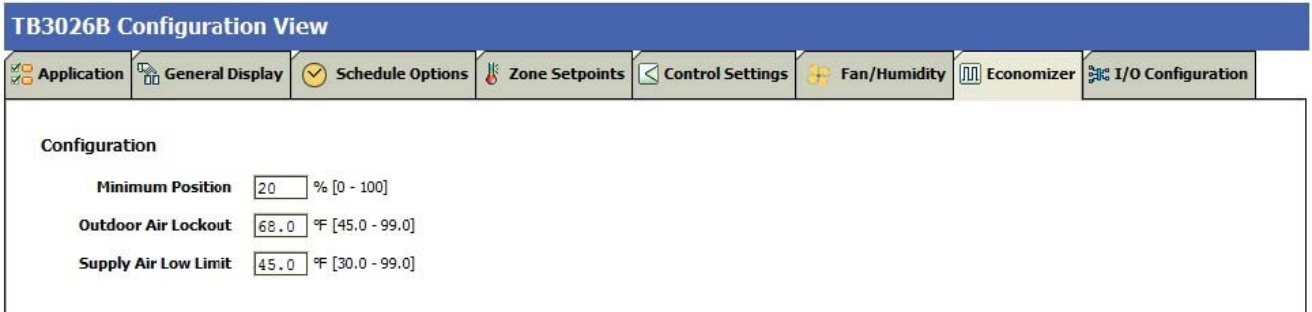
Fig. 50. Economizer Screen (Air Source Heat Pump)
