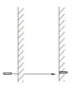
Step 2: Pinpoint the positions on the wall then drill four holes accordingly and fix the wallplugs into the wall.
