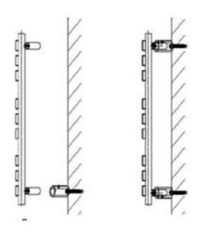
Step 5: Mount the towel rail to the wall and tighter the crews in the brackets.
