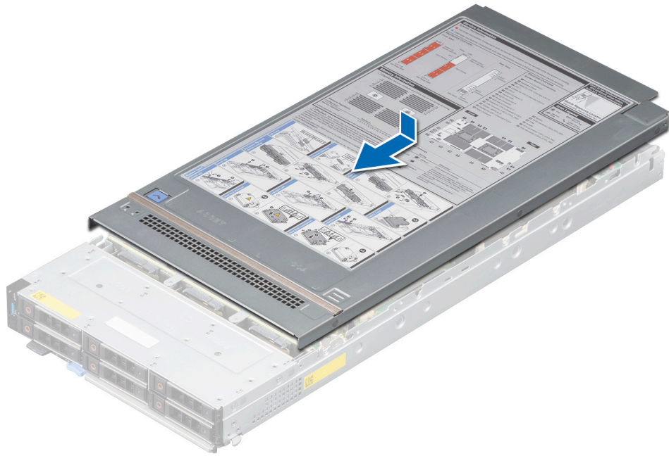
Figure 16. Installing the sled cover
