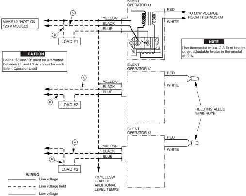
Typical Wiring Diagram To "Sequence" Two Or More Loads
