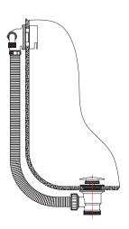
5. Tighten screw plastic nut to the waste body, and put back cover;
