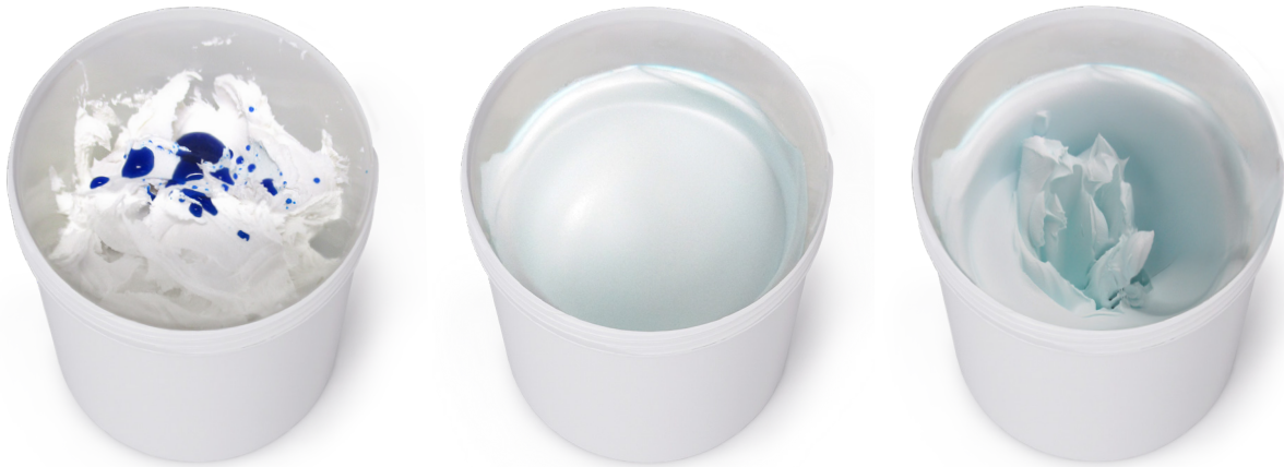
Figure 3. Mixing process using the gako PM140.
