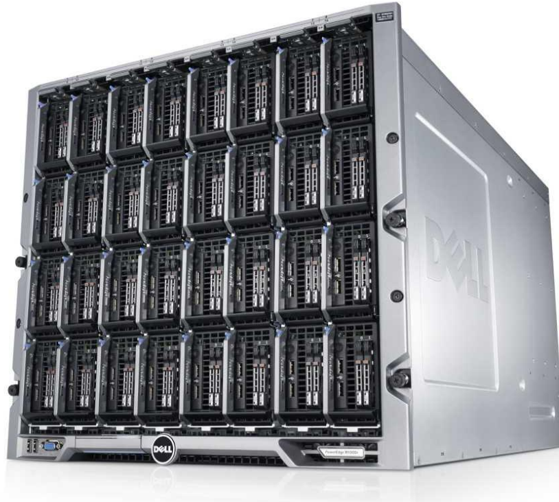
Figure 3. M1000e chassis enclosure with 32 M420 blades
