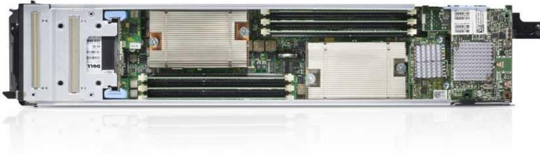
Figure 4. M420 internal module view
