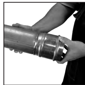
Figure 9: Inspection of final crimp
