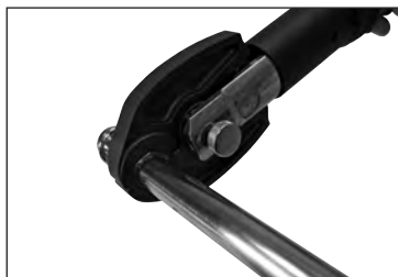
Figure 7 — Open the jaw set and place around the fitting
