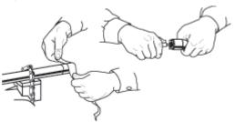
4. Apply flame to the fitting to heat tube and solder cup of fitting until solder melts when placed at joint of tube and fitting.
