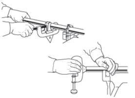
3. Apply solder flux to outside of tube and inside of cup of fitting carefully so that surfaces to be joined are completely covered. **Use flux sparingly.**
