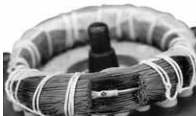
Fig. 40 PTC sensor incorporated in windings
