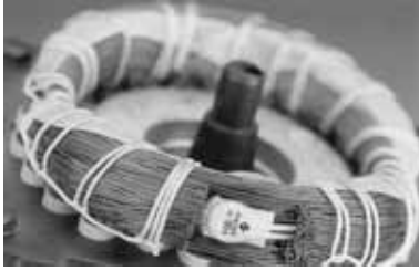
Fig. 42 Thermal switch incorporated in windings
