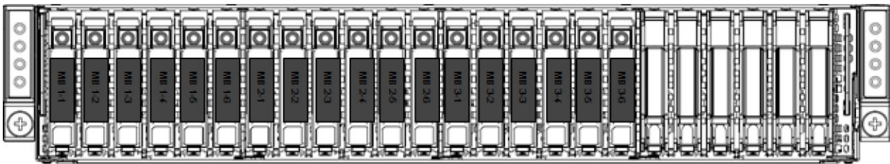
Figure 10. 2.5-inch drives (24) with three C6520 sleds
