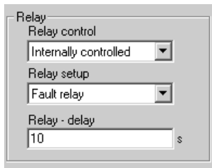
Fig. 20 Signal relay parameters for 0.5 - 10 HP pumps
