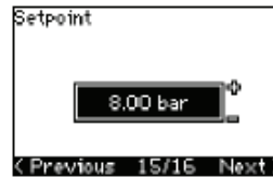
11. Enter setpoint pressure
