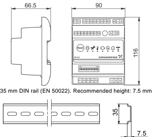
35 mm DIN rail (EN 50022). Recommended height: 7.5 mm
