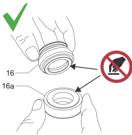
Fig. 18 How to correctly hold the shaft seal
