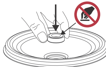
Fig. 20 Fitting the stationary part of the shaft seal
