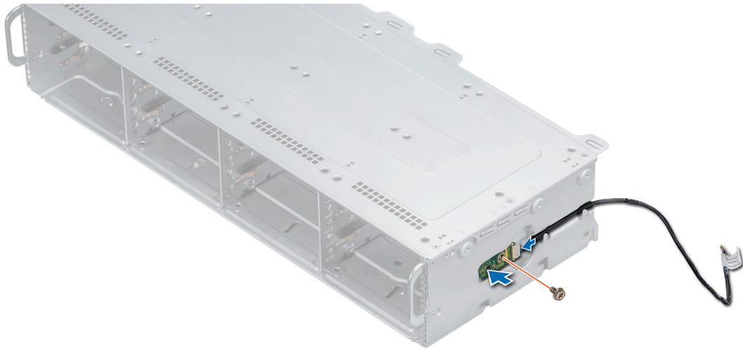
**Figure 70. Installing the sensor board assembly**
