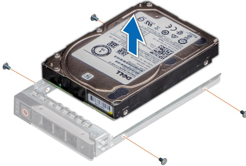
Figure 26. Removing the drive from the drive carrier
