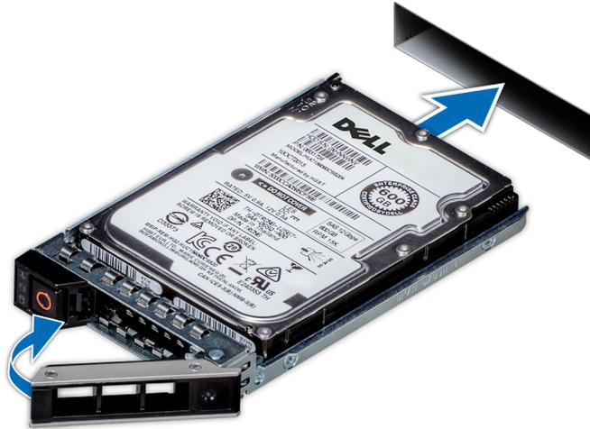
Figure 23. Installing a drive carrier
