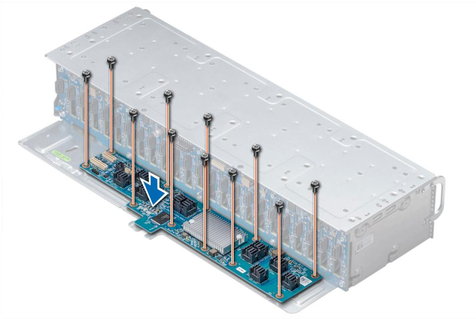
**Figure 64. Installing the backplane expander board**
