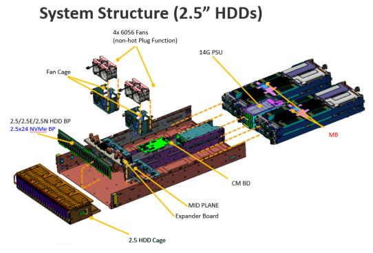
Figure 3. Inside the system C6400
