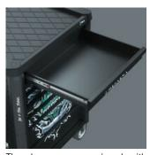
The drawers are equipped with ball bearing telescopic slides and can be pulled out completely. Selfclosing and mutually locking to prevent unintentional opening, thus minimal risk of tilting for roller cabinets. The carefully considered drawer design allows optimal use of the interior space. The dirtresistant drawer coating makes cleaning easy.
