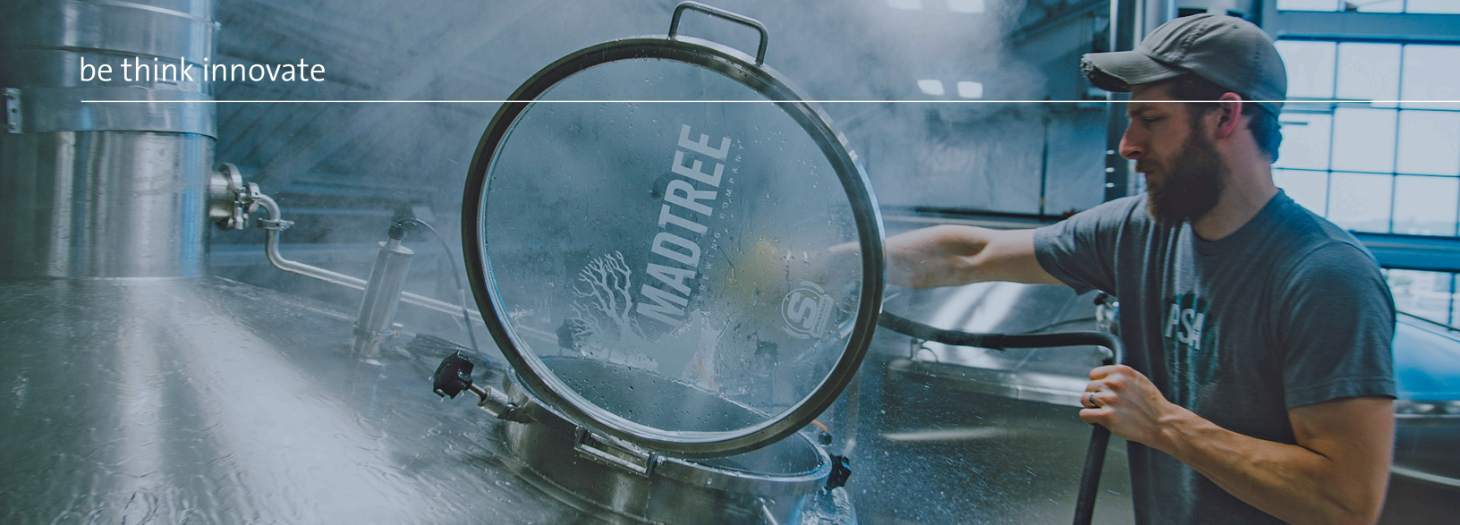
Above: Director of Brewing Operations, Matt Rowe, sprays out the mash / lauter tun on MadTree's 126 BBL production brewhouse during a brew day.
