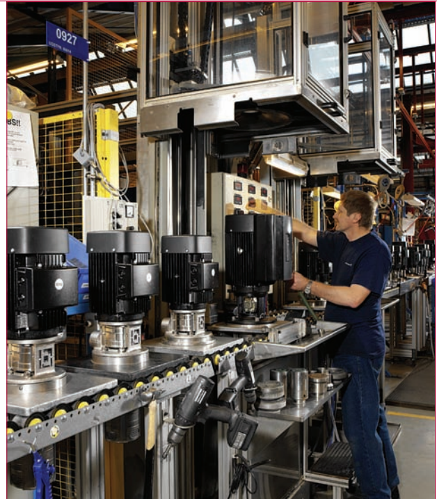
Assembly line of immersible pumps at Grundfos.
