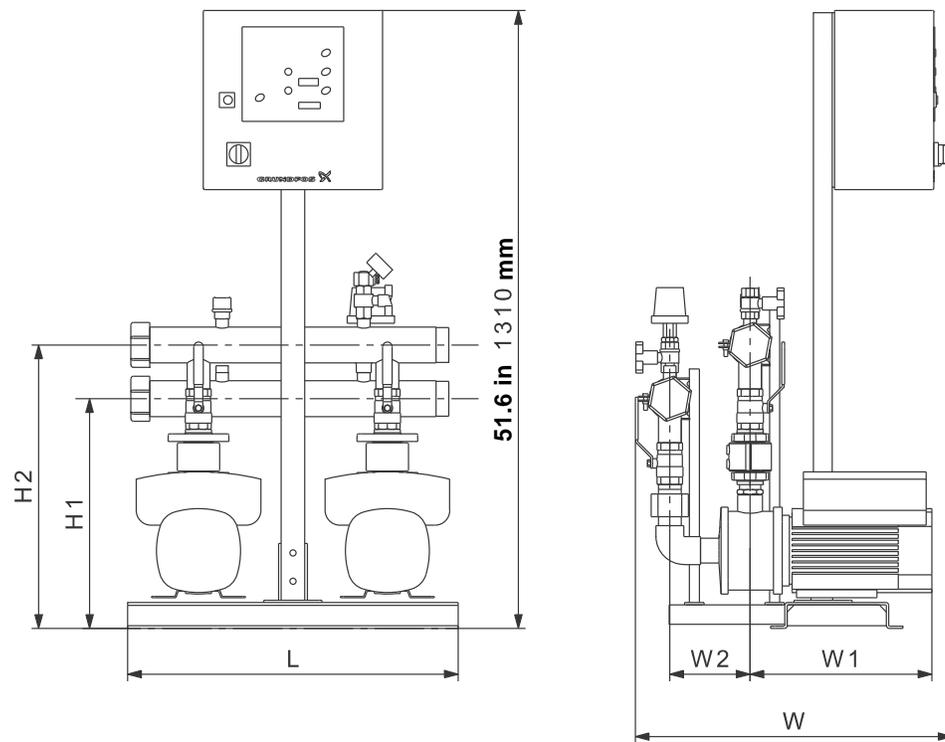
Fig. 13 Hydro Multi-B booster system with two CM, CME pumps
