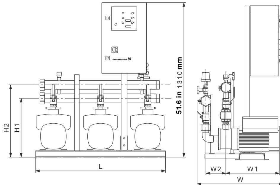
Fig. 12 Hydro Multi-B booster system with three CM, CME pumps
